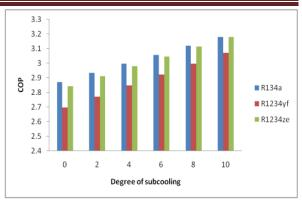
Fig: 4. Variation of COP with degree of subcooling at condenser outlet
