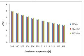
Fig: 6. Variation of COP with condenser temperature
