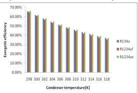
Fig: 7. Variation of exergetic efficiency with condenser temperature
