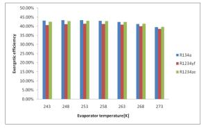
Fig: 2. Variation of exergetic efficiency with evaporators' temperatures
